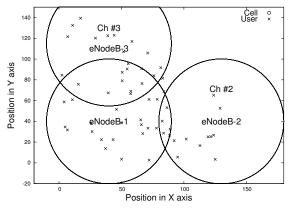
Fig. 1: An example of LTE-U network with three overlapping eNodeBs.
