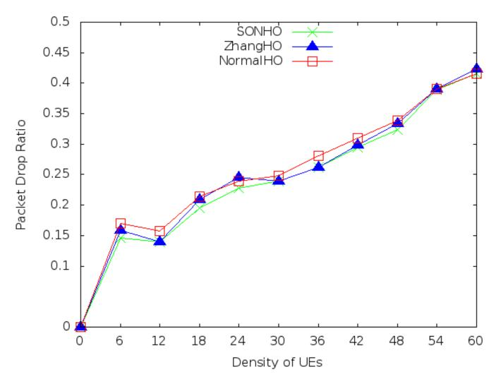
Packet drop ratio during handovers is less when SON algorithm is employed
