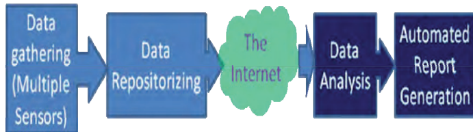
Figure 4. The flow diagram of the entire system including the network performance measurement, analysis, and automated documentation process.
