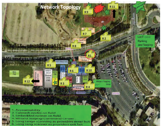
Figure 1. Topology of the deployed WMN (WMN routers are numbered from R1 through R12).
