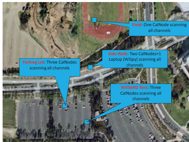
Figure 2. Location of CalNodes for non-invasive network performance measurement during Operation Golden Eagle.
