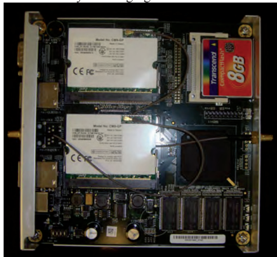
Figure 3. Inside view of traffic sampling node, CalNode.
