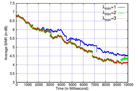
Fig. 8: Average SINR of all users in the network over 10 sec with mobility and varying  $\lambda_{min}$ .
