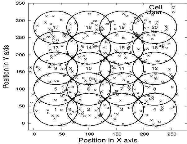
Fig. 3: Positions of 20 eNodeBs with 400 UEs in small cell network.
