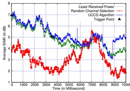
Fig. 7: Average SINR of all users in a cell over 10 sec with mobility.
