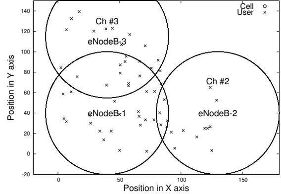
Fig. 1: An example of LTE-U network with three overlapping eNodeBs.
