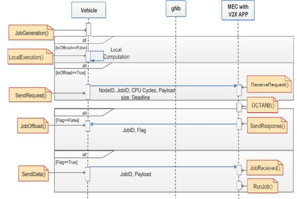
Fig. 2: Sequence Diagram of UdpOffloading Application.
