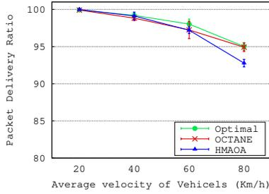
**Fig. 6:** PDR Vs velocity of vehicles for  $V = 30$ .
