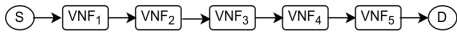
Figure 2: Example of sequential SFC request. S and D represent the source and destination, respectively.
