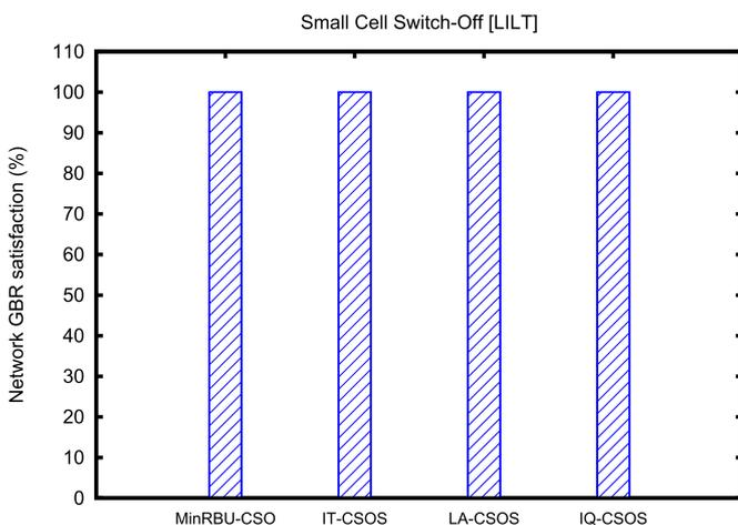
**Fig. 17.** Scenario #2: Comparison of GBR satisfaction in various CSOSs. The plot shows that irrespective of interference in the HetNet during low traffic load contrast to other CSOSs, the IQ-CSOS could switch-off more small cells and also ensures higher GBR satisfaction to UEs.
