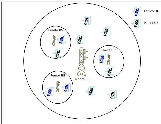
Fig. 1. A simple LTE-HetNet deployment.
