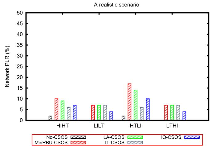
Fig. 22. Scenario #3: Network condition is varied from HIHT to LTHI, and observed PLR is plotted in various CSOSs. In a given HetNet, irrespective of interference during low traffic the IQ-CSOS is causing 4% of PLR and during high traffic the IQ-CSOS is causing 10% of PLR. During high traffic, because of interference other CSOSs are causing around 15% of PLR.
