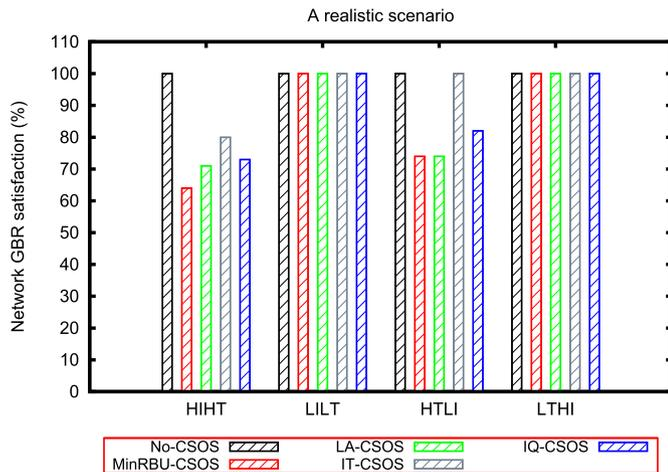
Fig. 21. Scenario #3: Network condition is varied from HIHT to LTHI, and observed network GBR satisfaction is plotted in various CSOSs. In a given HetNet, irrespective of interference during low traffic the IQ-CSOS ensures 100% of GBR satisfaction to UEs and during high traffic the IQ-CSOS ensures 80% of GBR satisfaction to UEs. During high traffic, because of interference other CSOSs could be able to ensure only around 65% of GBR satisfaction to UEs.
