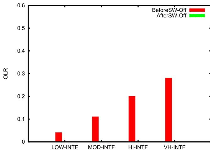
Fig. 9. Variation in OLR of Macro eNB for different interference levels: the plot shows that CSO can decrease interference in the network and reduces network OLR.
