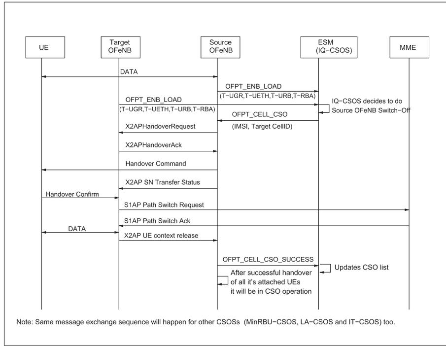
Fig. 5. Call flow diagram of CSO in SD-LTE-RAN framework.
