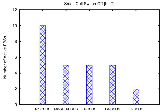
Fig. 15. Scenario #2: Comparison of number of active FBSSs in various CSOSs. The plot shows that irrespective of interference in the HetNet, the IQ-CSOS is able to switch-off more small cells compared to other CSOSs.
