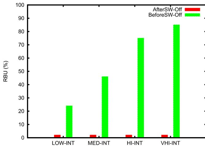
Fig. 8. Variation in RBU of Macro eNB for different interference levels: the plot shows as interference increases in the HetNet, the RBU of Macro BS also increases.
