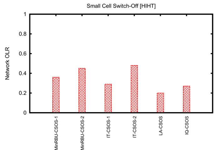
**Fig. 12.** Scenario #1: Comparison of network OLR in various CSOSs. The plot shows how network OLR is affected by various CSOSs. LA-CSOS and IQ-CSOS are considering network overload into CSO decision, hence they are able to maintain network OLR around 0.2.
