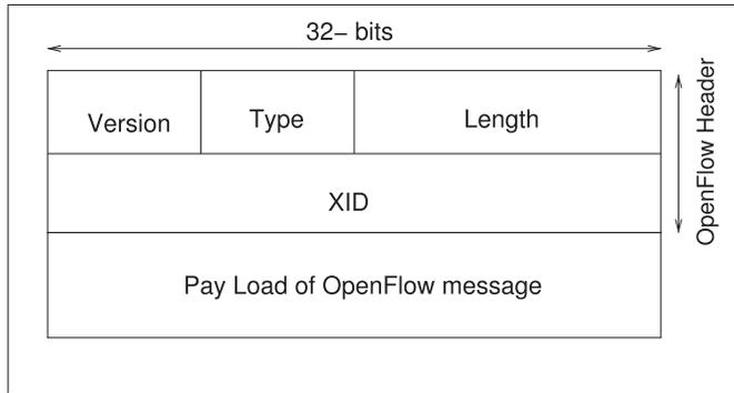
Fig. 6. Frame format of OpenFlow LTE messages.
