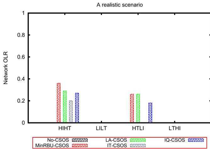
Fig. 20. Scenario #3: Network condition is varied from HIHT to LTHI, and observed network OLR is plotted in various CSOSs. In a given HetNet, irrespective of interference during low traffic the IQ-CSOS ensures network is not overloaded and during high traffic the IQ-CSOS ensures network overload is around 0.2. During high traffic, because of interference other CSOSs could be able to ensure network OLR around 0.35 only.
