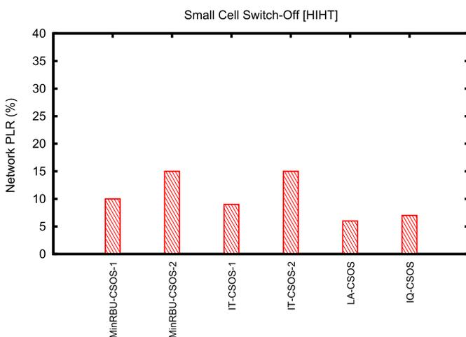
Fig. 14. Scenario #1: Comparison of PLR in various CSOSs. LA-CSOS and IQ-CSOS are considering network overload into CSO decision, hence they are causing lesser packet losses compared to other CSOSs.
