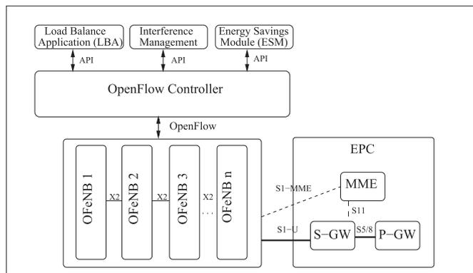
Fig. 4. Architecture of SD-LTE-RAN (Rangiseti Tammaet al., 2016).
