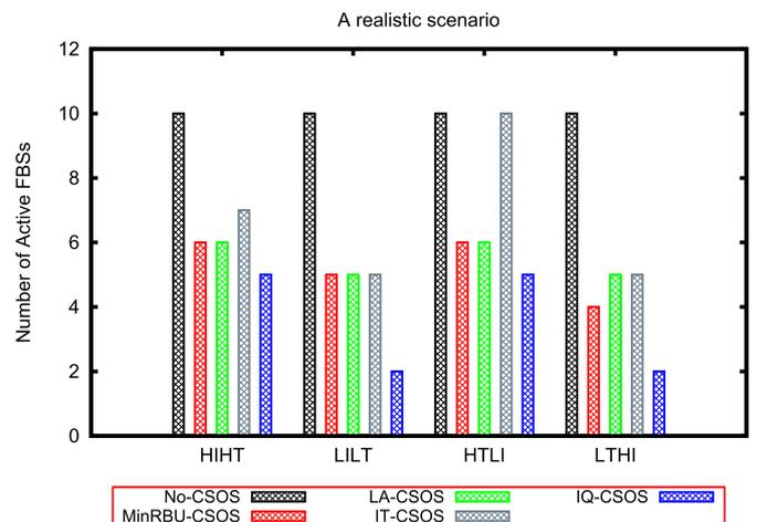
**Fig. 19.** Scenario #3: Network condition is varied from HIHT to LTHI, and observed number of active FBSs is plotted in various CSOSs. In a given HetNet, irrespective of interference during low traffic the IQ-CSOS needs only 2 ActBSs and during high traffic the IQ-CSOS needs 5 ActBSs. But, other CSOSs need 5 to 7 ActBSs based on traffic load.
