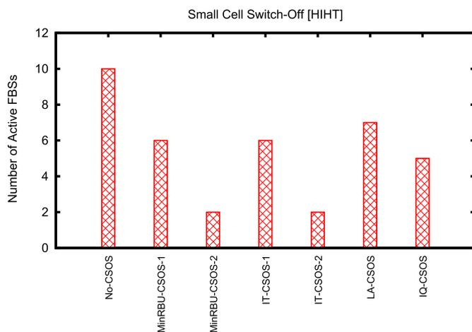
**Fig. 11.** Scenario #1: Comparison of number of active FBSs in various CSOSs. The plot shows number of ActBSs needed by CSOSs to handle HIHT. Since IT-CSOS and IQ-CSOS are considering the interference in the HetNet, they are able to switch-off more FBSs.
